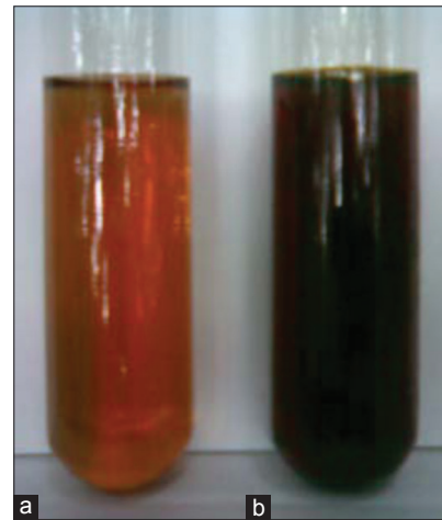
Figure 1: Mangifera indica leaves extract (a) before and (b) after the formation of silver nanoparticles
